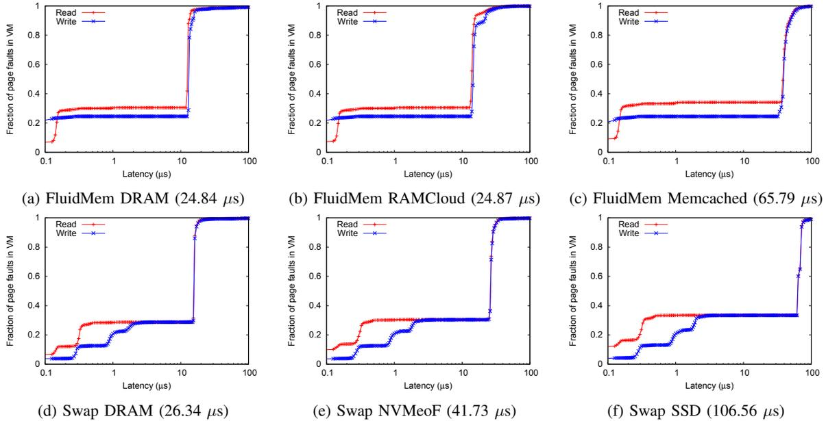
Figure 3: CDF of latencies measured with pmbench. The plots are arranged row-wise by mechanism (FluidMem vs. Swap). Average latencies for each backend are shown in parenthesis.
