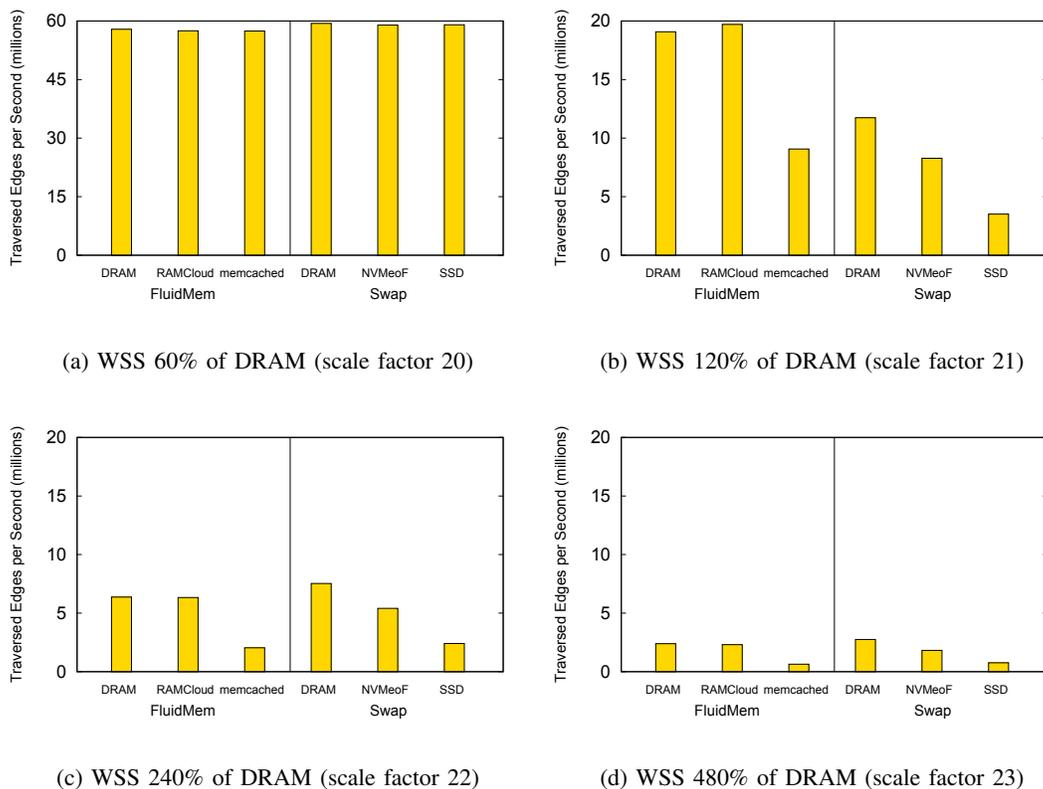
Figure 4: Graph500 performance with working set sizes (WSS) from 600 MB (scale factor 20) to 4.8 GB (scale factor 23). The overhead of FluidMem page faults is 2.6% in (a). The benefit of storing OS pages in remote memory with FluidMem is most pronounced in (b) when WSS is 120% of DRAM. At higher scale factors (c) and (d), the performance of FluidMem RAMCloud exceeds swap to NVMeoF, but choices in page eviction penalize FluidMem DRAM compared to swap.
