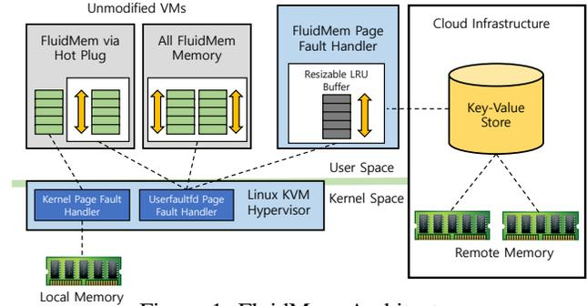
Figure 1: FluidMem Architecture
