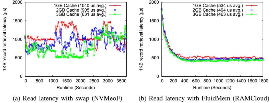
Figure 5: Latency of YCSB 1 KB read-only workload for MongoDB with WiredTiger storage engine. When cache size exceeds DRAM capacity, the storage engine is not capable of achieving a stable working set when only given swap space via NVMeoF. When remote memory performance is comparable (Figure 3), FluidMem achieves significantly lower average latencies because it transparently provides the storage engine with native memory capacity.
