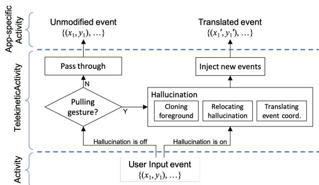
Figure 2: Input event flow inside TelekineticActivity.
