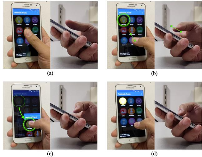
**Figure 1:** (a) Some icons are out of the thumb's reach. (b) User performs a pulling gesture above the screen. (c) The entire application screen relocates closer to the thumb location. (d) Clicking an icon on the relocated screen is applied to the original application.
